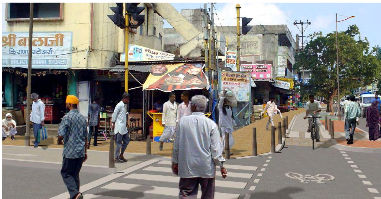
Optimum utilization of existing roads by insertion of cycle tracks and zebra crossing
