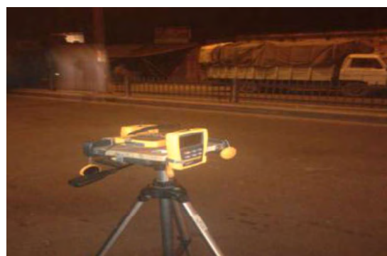
Figure 52: Assembly of 3 light meters mounted on a tripod.
