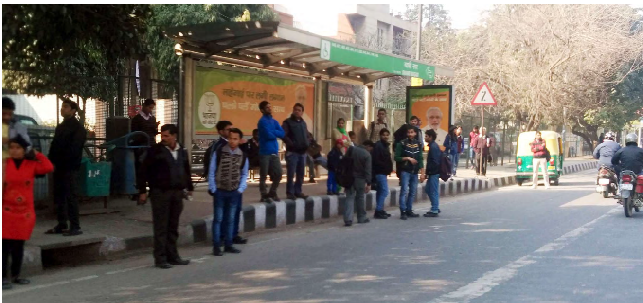
No buffer space for a bus-stop located on a major arterial road, makes the waiting passengers exposed to fast moving traffic, thereby creating high risk, unsafe situations. Location: Outer Ring Road, Delhi. Source: Authors
