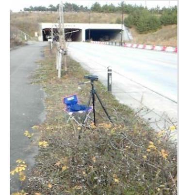
Upstream camera (showing dummy radar gun)
