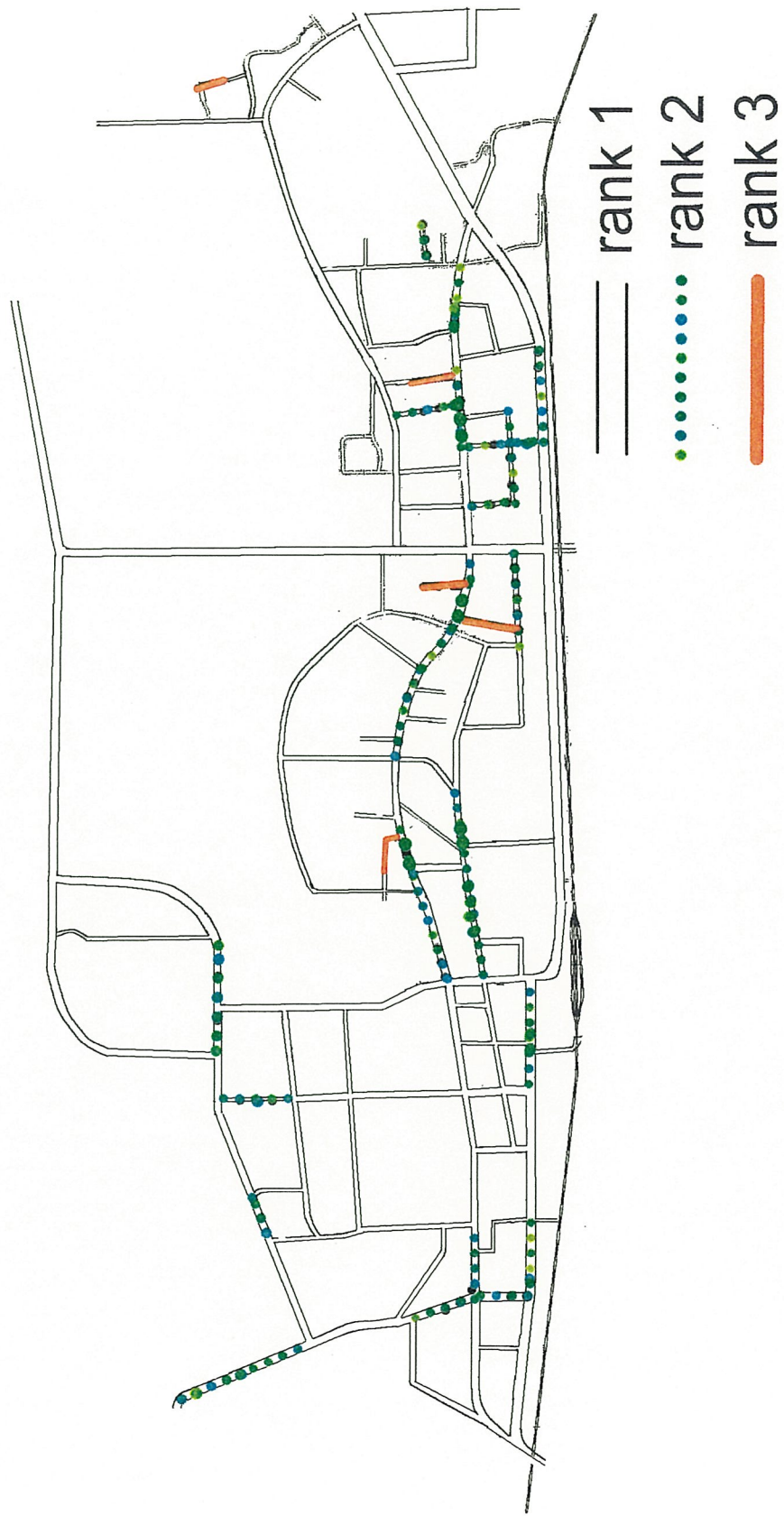
Figure 3-3 Street damage based on on-site surveys in Chi-Chi
