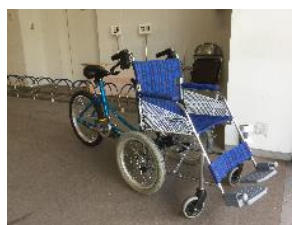
Three-wheeled bicycle with wheelchair
