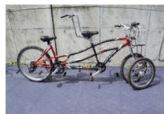
Double front-wheel tandem
