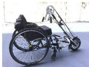
Three-wheeled handcycle with wheelchair
