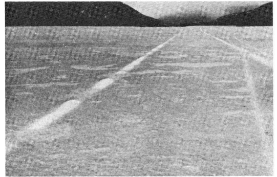
Fig. 13 ピーター湖の氷上に着陸した DC-3 の車輪の摩擦痕 The surface of Peters Lake showing patches of c-axis-vertical ice in the c-axis-horizontal ice (the tack of a taxing DC-3 airplane)
