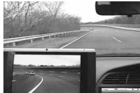
Fig. 11 Movie transmission over inter-vehicle communications with 5.8GHz DSRC in 2004
