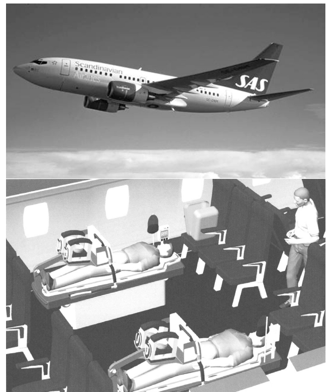
Fig. 6 Swedish National Medevac. Within six hours, a regular SAS passenger aircraft can be converted to transport six intensive care patients and a further 20 more or less severely injured. (Photo published with courtesy of MICUS AB and SAS)
