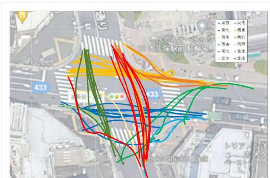
Trajectory of electric scooters near/at the intersection
