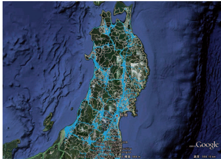
Figure 8. Example of probe information system (Honda Internavi traveling experiences immediately after the Great East Japan Earthquake) 9)
