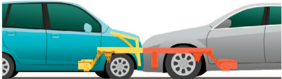
Figure 3. Schematic diagram of crash-compatible car bodies 2)
