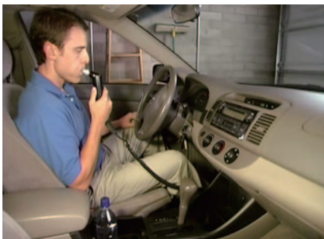
Figure 2. Ignition interlock device
