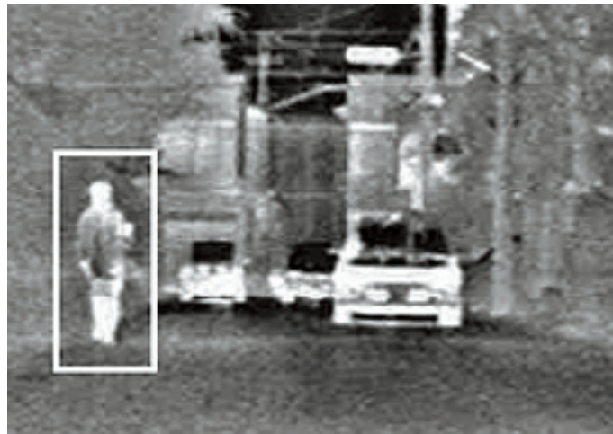
Figure 2. Intelligent night vision system enhancing visibility of pedestrians 1)
