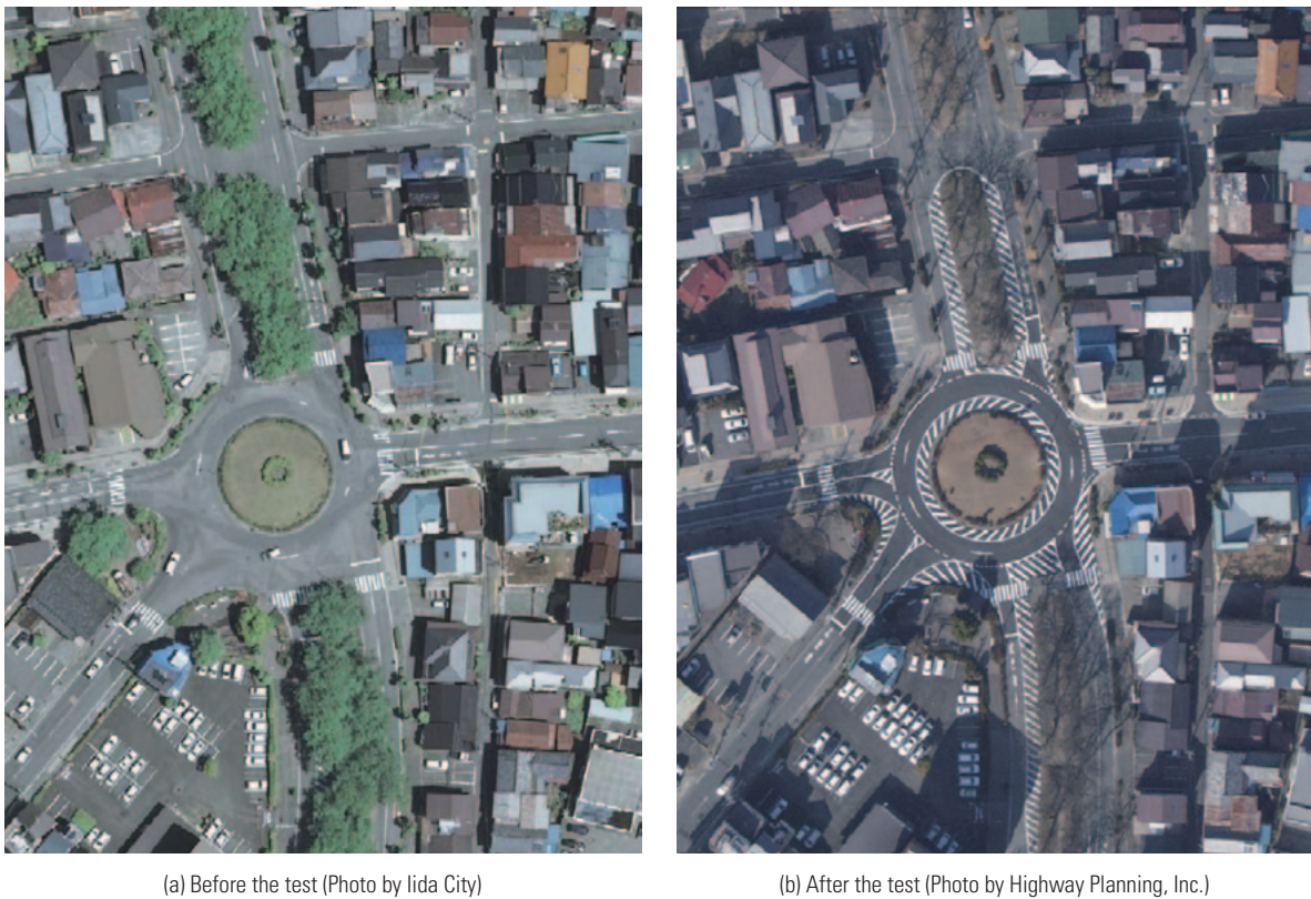
Figure 1. The roundabout on which field operational tests were performed in 2010; Azuma-cho, Iida City, Nagano Prefecture
